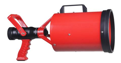
The T series medium expansion foam nozzle is a kind of oil fire fighting equipment. The all-metal material design can be used for a long time in harsh environments. The foam nozzle is composed of nozzle, handle, barrel,quick connect, etc., suitable for various mixing ratios, and can ensure effective spray distance. Advanced surface treatment technology ensures long-term corrosion resistance.
